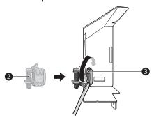
Insert the electrical cable through the hole in the strain relief. Tighten 2 screws to secure the cable.
