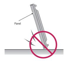
2 If the product is tilted toward the corner of the panel, the bottom of the panel may be damaged.
