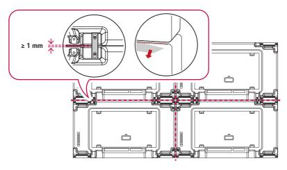
3 Complete the 2 x 2 tiling. You can use various options of tiling including 3 x 3 by using the same method.
