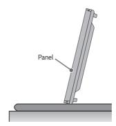
2 When laying down the product, lay a cushion on a flat floor. Put the product on it with the panel of the product facing down.
