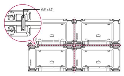
2 Adjust the spacing between the sets using the tiling guide, and remove the protective sheet.
