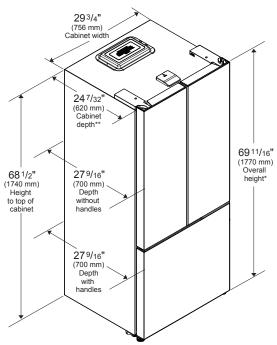
\*Add 1" (25.4 mm) with front leveling feet fully extended \*\*Add 13/16" (30 mm) for spacers on back
