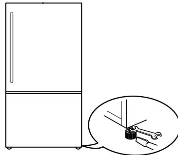
**2** Open both doors, and check to make sure that they close easily. If the doors do not close easily, tilt the refrigerator slightly more to the rear by turning both leveling legs to the left. It may take several more turns, and be sure to turn both leveling legs the same amount.
