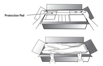
2 To stand the product upright, hold it on both sides so that the LED package screen does not touch the floor.
