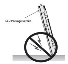
2 If the product is tilted towards the edge of the LED package screen after the brackets on the corners are removed, the bottom (corner) of the product may be damaged.
