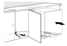
Remove the tape from the water supply line and the electrical cable.
