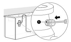
Remove the knockout plug 1 from the disposal.
