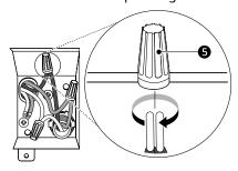
Wrap electrical tape 6 around each connection.
