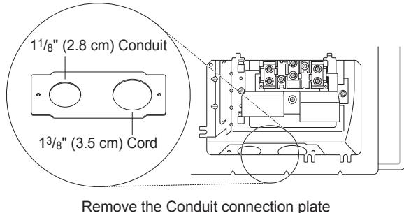
Remove the Conduit connection plate
