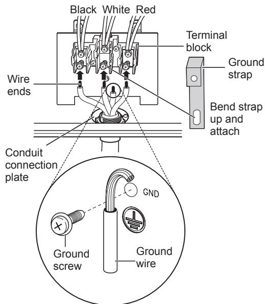
If screws are not tightened securely, it can result in electrical spark and severe personal injury or death.
