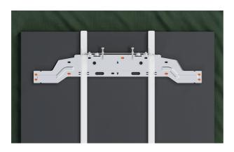
**9.** Secure the bracket to the panel using the four small screws from the side gauges and three screws from the install kit. Drill pilot holes before fixing the screws.
