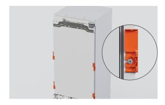
1. Loosen the screws and slide the four door panel brackets onto the refrigerator door. Tighten to secure.
