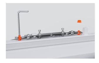
2. Remove the nuts, then raise the door panel hanging brackets by 3/16" (5 mm) using an Allen key.
