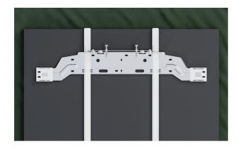
7. Place the bracket on the back of the panel with the height gauges hooked over the top edge.
