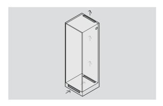
2. Ensure the alcove is square, has a finished return, and includes a ventilation cutout through the plinth and out of the cavity. Avoid venting directly into the adjacent cabinetry.
