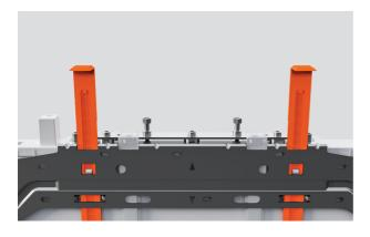
**3.** Pull the height gauge up to remove it, flip it front to back, and reinsert it into the adjacent slot. Adjust the gauge until it clicks into the correct position.
