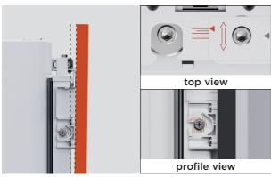
**3.** Adjust panel tilt using the side door brackets.
