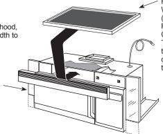
Filter Kit WB02X35607 (included) Recirculating Charcoal Filter Kit To be used when the microwave oven cannot be vented to the outside.
