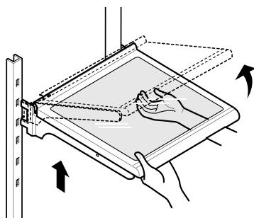
**5** To assemble, tilt the front of the shelf up and guide the shelf hooks into the slots at a desired height.
