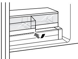
**6** Line up the tabs on the Door-in-Door case with the slots on the door and push down until it snaps into place.
