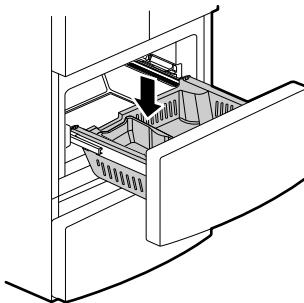
**2** Grasp the drawer on each side and hook the drawer supports into the rail tabs located on both sides.
