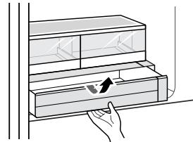
**2** To assemble, slightly tilt up the front, insert the drawer into the frame and push it back into place.
