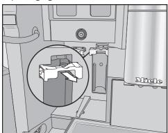
Pull the descaling cartridge holder forward.
