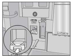
Pull the cleaning cartridge holder forward to remove it.
