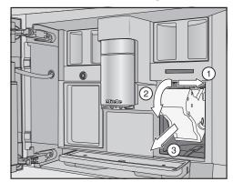
■ Pull the brew unit to the side ① first and then pull out to the front ②. Tilt the brew unit forward ③.
