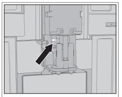
Do **not** remove the milk pipework connecting piece.
