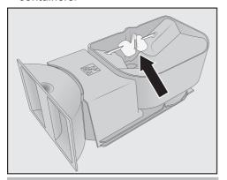
Do not remove the components for improving the flow of the beans (see arrow).
