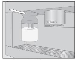
Push the milk flask back into the coffee machine until it clicks into place.
