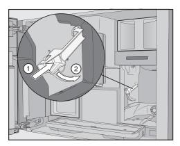
■ Press the button under the handle of the brew unit ① and, while doing so, turn the handle backward ②.
