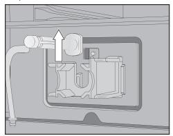
Pull the stainless steel bolt upward and out.
