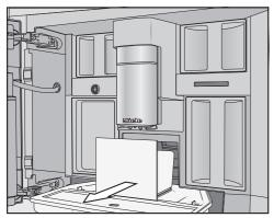
Remove the drip tray and grounds container from the machine. ■ Empty the grounds container after removing it from the drip tray.
