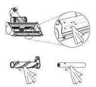
Slide the brushes back into the nozzle and rotate the cover back into place. Turn the cover lock clockwise to lock the cover.
