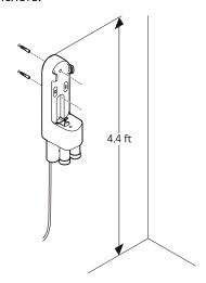
**3** Attach the charging station to the wall with the wall anchoring screws.
