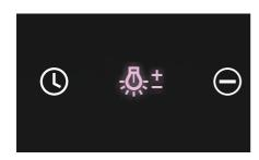
With range hood OFF, press and hold Lights button until adjacent buttons flash red for WARM or white for COLD.
