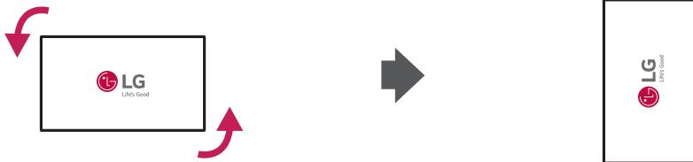
When installing vertically, rotate the monitor 90 degrees clockwise while facing the front of the screen.
