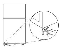
**2** Open both doors, and check to make sure that they close easily. If the doors do not close easily, tilt the refrigerator slightly more to the rear by turning both leveling legs to the left. It may take several more turns, and be sure to turn both leveling legs the same amount.
