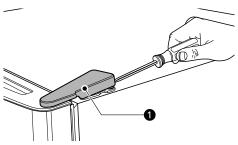
Using a 10 mm or 3/8 inch socket wrench, remove the three bolts and lift the top hingeSet the parts aside.
