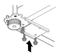
2 Move the leveler 1 to the opposite side of the housing, keeping the same orientation, and reattach it with the 2 bolts removed earlier.
