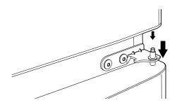
Place the top hinge on top of the freezer door and line up the hinge with the holes on top of the refrigerator. Use the three bolts to fasten the hinge.
