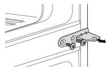
4 Using a 1/4 in. socket wrench, loosen and remove the bottom hinge pin 4 from the bottom hinge bracket 5.
