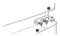
Lift up the refrigerator door slightly and remove it. Set the door aside on a nonscratching surface.
