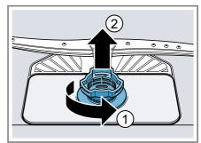
Pull the micro filter downward and off.
