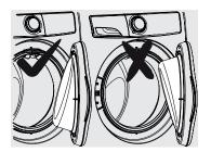
Plug in washer and close the door. Test correct door lock operation by starting a test cycle: lock should engage, and door should not be able to be opened until cycle is paused or canceled.
