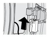
2. Slide terminal cap onto back of hinge plate until tabs snap into place.
