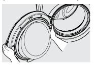
While supporting the door with one hand, pinch the tabs to release the plastic terminal cap from the hinge plate.
