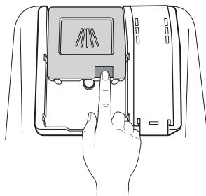
**2** Add dishwashing detergent to the main wash compartment until the level is between the lines marked 15 and 25.
