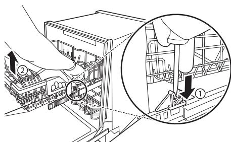
**3** To remove the back rack supports from the rails, hold a side rail with one hand, lift the front of the rack, and firmly push the rack back to snap the support out of the hooks in the rear. Repeat on the opposite side.
