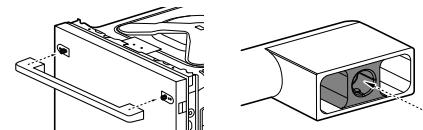
**3** Fit the new handle over the mounting fasteners as shown and tighten the set screws to secure it in place.
