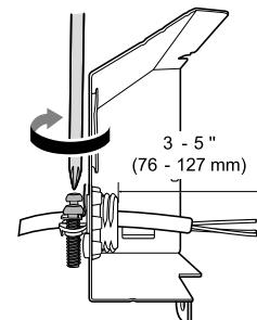
**7** Pull the existing wires through the openings in the junction box. Tighten 2 screws **④** to reassemble the junction box in the appliance.
