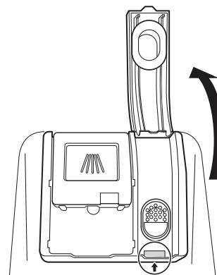
**2** Add a liquid rinse aid to the maximum fill level. Allow the rinse aid to settle in the dispenser while filling, or air bubbles may
