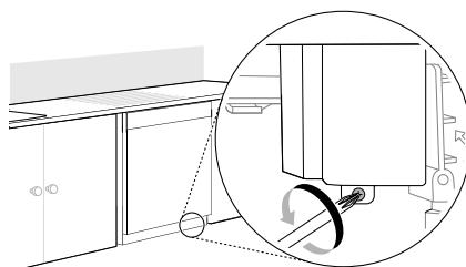
**3** Use a Phillips screwdriver to remove 2 screws **①**.
