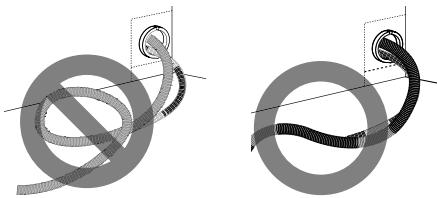
**4** Gradually slide the dishwasher into the opening, making sure that the water supply line and electrical cable are passing freely through the channels and do not get caught under the dishwasher.
