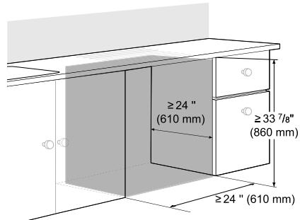
**2** To allow for proper clearance of plumbing and electrical, use the template included with the literature to determine the clearance on the side of the cabinet where the cabinet meets the back wall. Using a 2 1/2" diameter hole saw, drill a hole in the target area as shown.
