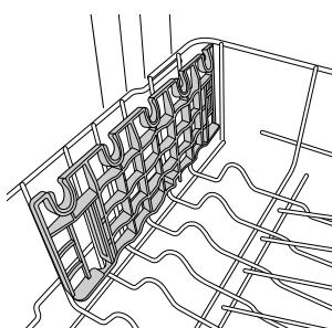
**2** Locate the assembly slot ① on the cup rack, align the slot with the bar, and firmly pop the rack off the support bar on that side.
