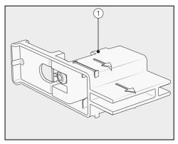
■ Do **not** remove the installation aids ① from the appliance door. These will be required later for aligning the appliance in the installation niche.
