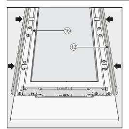
■ Now insert the angle trims <sup>13</sup> on both sides as far as they will go into the provided spaces in the mounting frame <sup>16</sup>.
