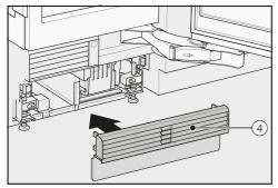
■ Click the toe-kick ventilation grille ④ onto the bottom of the appliance toe-kick.
