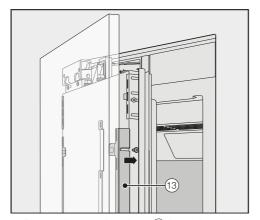
Press the angle trims <sup>®</sup> into the white plastic frame on both sides and screw them on loosely at first. Spare screws are provided in the plastic bag marked with the letter E.
