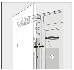
■ Align the depth of the cabinet front via the gaps in the angle trims <sup>13</sup>.
