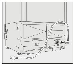
Insert the electrical plug into the back of the wine storage unit.
