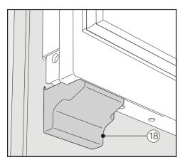
■ Click the covers <sup>18</sup> onto the fixing brackets.
