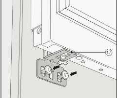
■ Screw the fixing bracket <sup>17</sup> securely to the cabinet front.
