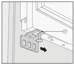
■ Slide the fixing bracket ⑰ from the outside onto the screw at the bottom of the appliance door.
