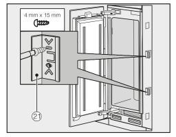
■ Secure both sides of the wine conditioning unit using at least 3 clips ② for the covers.
