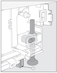
■ Position the supplied spacers ⑦ on both sides on the markings next to the adjustable feet at the front of the wine conditioning unit.
