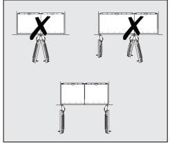
If the wine conditioning unit/appliances are to be installed next to each other without a partition wall between them, they will need to be joined together with the side-by-side merging kit. In addition, you must install the heating mat to prevent condensation from forming and any resulting damage.
