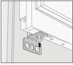
■ Tighten the screw at the bottom of the appliance door.
