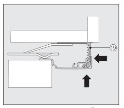
Place the assembled cover <sup>(9)</sup> into the gap above the wine conditioning unit so it clicks into place. While doing so, slide both parts of the cover together as required.
