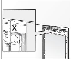
■ Measure the gap **X** between the mounting frame and the upper edge of the adjacent cabinet front.
