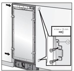
■ Screw the retaining plate lugs <sup>12</sup> at the top and bottom to the cabinetry adjacent to the appliance.
