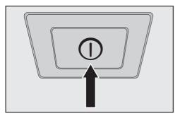
Switch the wine storage unit on by pressing the On/Off switch.
