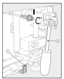
■ Adjust the rear feet with a ratchet (attachment: socket, 8 mm) or a TX 20 screwdriver ⑧.
