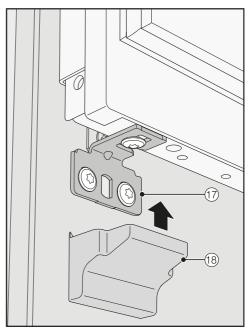
■ Install the cover <sup>18</sup> over the fixing bracket <sup>17</sup>.
