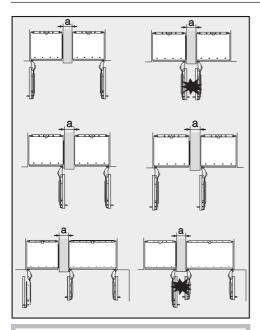
If the door hinges of the appliances are next to each other, you must take into account the thickness of the cabinet fronts and door handles so that the appliance doors do not collide and become damaged if they are opened at the same time.
