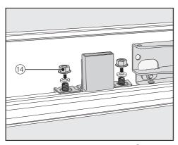
■ Place the washers and nuts <sup>(1)</sup> back in position and tighten the nuts <sup>(1)</sup>. The cabinet front is now secured.
