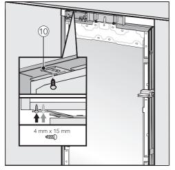
Screw the lugs for the retaining plate
