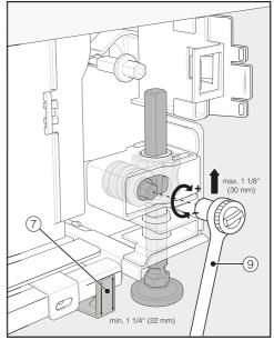
■ Adjust the front feet with a ratchet (attachment: socket, 8 mm) or a TX 20 screwdriver ⑨.
