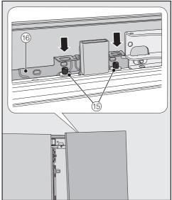
■ Open the appliance door and hang the cabinet front on its frame <sup>16</sup> onto the threaded bolts <sup>15</sup>.
