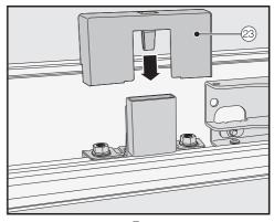
■ Install the cover ② onto the light contact switch.
