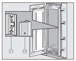
■ Now attach the covers ② onto the retaining clips ② on both sides.
