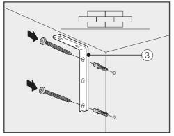
Securing to a concrete wall
