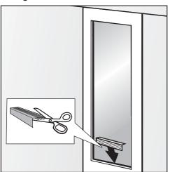
Cut the door trim to the width of the cut-out in the cabinet front as required. An extra length of trim is supplied to help calculate the length required.
