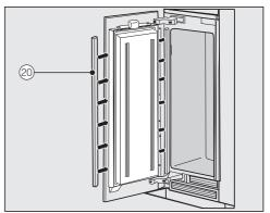
■ Install the two plastic covers <sup>20</sup> on both sides of the appliance door by clicking them into the gap between the appliance door and the cabinet door, starting at the bottom and working up to the top.
