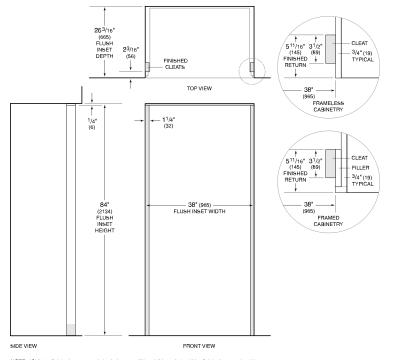
NOTE:  $3^1y_2^{\prime\prime}$  (89) finished returns and shaded areas will be visible and should be finished to match cabinetry. Shaded line represents profile of unit with  $3^1/4^{\prime\prime}$  (19) panel.
