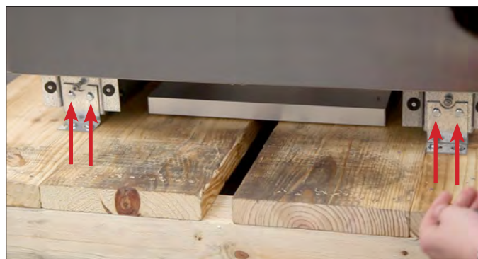
FIG. 7. Shipping bracket bolt locations.
