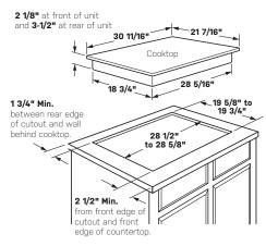
To ensure accuracy, it is best to make a template when cutting the opening in the counter.
