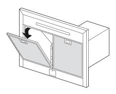
• To reassemble the filter, insert the back of the filter first and then lift the filter up into place.
