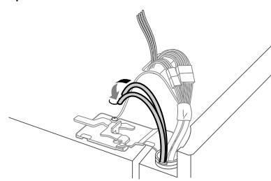
**4** Push the water supply lines into the hole on the top case and pull them through the backplate.
