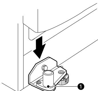
**2** Fit the hinge **2** over the hinge lever latch **3** and slot it into place. Rotate the lever **4** clockwise and fasten the hinge.
