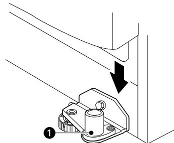
**2** Fit the hinge ② over the hinge lever latch ③ and slot it into place. Rotate the lever ④ counterclockwise to secure the hinge.
