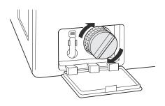
Close the drain pump filter cover.
