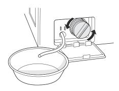
**5** Clean the pump filter and opening.
