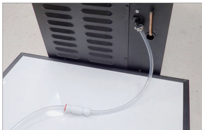
FIG. 5. Installed check valve.
