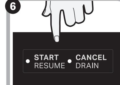
**Start / Resume Cycle. Close the door within 4 seconds for top control models.**
