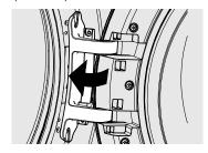
Reinstall all four screws removed earlier
