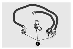
Rubber washer must be present and undamaged. 4. If your installation has room for the COLD water supply to accept the "Y" connector directly, thread the "Y" connector to the COLD water supply and snug it by hand; then tighten it another 2/3 turn with pliers.
