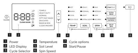
These temperature, spin speeds, soil levels and options are available with the following cycles:
