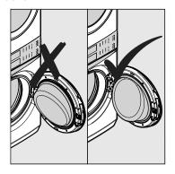
Plug in washer and close the door. Test correct door lock operation by starting a test cycle: lock should engage, and door should not be able to be opened until cycle is paused or canceled.
