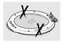
Lift the metal ring and rotate it 180 degrees, setting it back on the inner frame. Ensure gasket has not separated from the metal ring.
