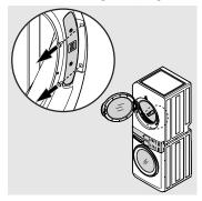
Remove both screws from door latch. Save latch and screws for reinstallation later.
