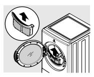
2. Press down the button on the top of the filter to open the clamshell.
