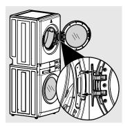
Reinstall and tighten all four screws removed earlier - two front screws first, then the two side screws.
