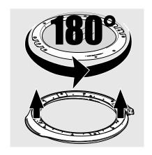
Make sure "THIS SIDE UP" AND "THIS SIDE DOWN" on the metal ring point in the corresponding directions.
