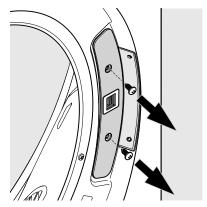
Locate and remove the screw holding the hinge cover. Save the screw and cover for reinstallation.
