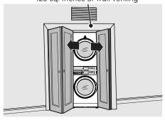
Solid Bi-Fold doors with no ventilation requires door open for 120 sq. Inches of wall venting
