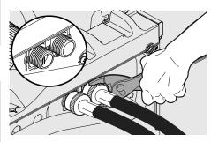
5. Connect the HOT inlet hose to the HOT water supply and the COLD inlet hose to the COLD water supply.
