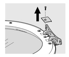
Locate and remove the two screws holding the striker. Save the screws and latch for reinstallation.
