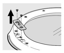
Remove remaining eight screws using a #2 square bit driver. Save the screws for reinstallation.
