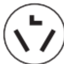
3-wire receptacle (10-30R)
