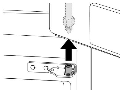
**3** Rotate the hinge lever **5** clockwise. Lift the top hinge **6** free of the hinge lever latch **7**.
