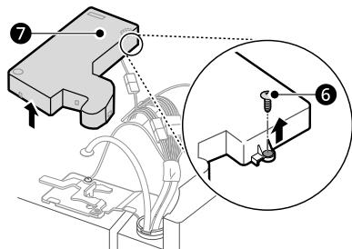
**3** Remove the cover and pull out the tube ⑧. Disconnect all wire harnesses ⑨. Unscrew the ground wire ⑩.
