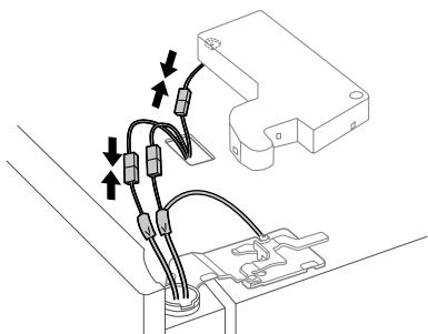
**4** Set the hinge cover **4** in place. Insert and tighten the cover screw **5**.
