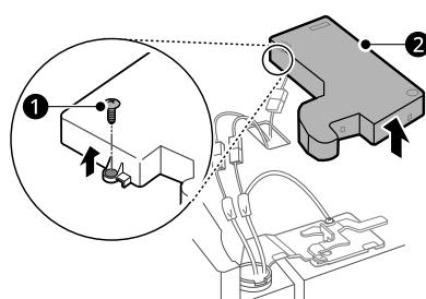
**2** Detach all the wire harnesses **3**. Unscrew the ground wire **4**. Remove the cover.
