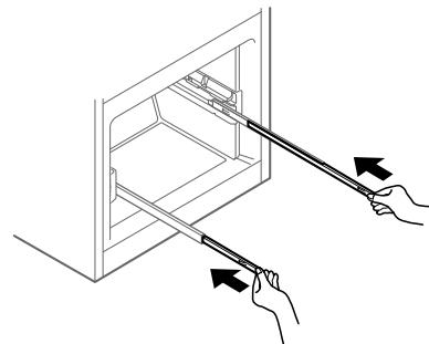
**4** Remove the Durabase basket from the rails. Remove the screws from the rails at both ends.
