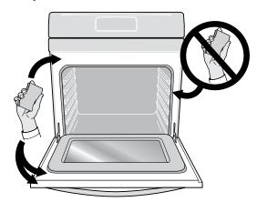
Figure 8: Clean around the oven door gasket
