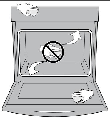
Figure 10: Do not clean oven door gasket
