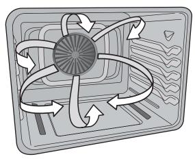
Figure 5: Convection roasting on lower oven racks
