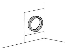
**3** Make sure the drain hose is straight before feeding the end of it through the hole for the water supply. As you slide the dishwasher into the opening, you will want to slowly pull on the drain hose from inside the cabinet to take up some slack. Be careful not to kink, pinch, crush or stress the drain hose during installation to avoid leaking and water damage.
