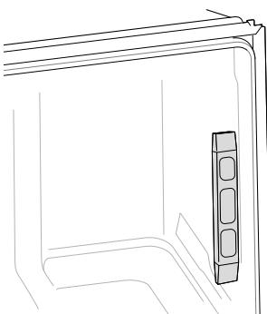
Make sure that the gap between the tub walls and the door liner is the same on either side.
