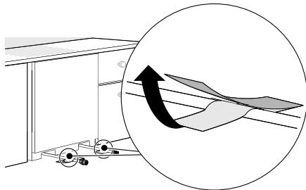
**4** Gradually slide the dishwasher into the opening, making sure that the water supply line and electrical cable are passing freely through the channels and do not get caught under the dishwasher.
