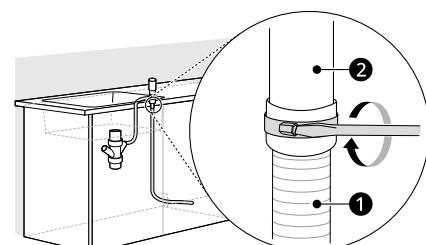
**3** If it is not connected, attach the rubber hose connector to the disposal or waste tee with a hose clamp (not provided).
