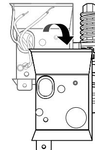
**5** Insert a 3/8" strain relief **2** through the hole in the junction box. Tighten the ring nut **3** to secure it in place.
