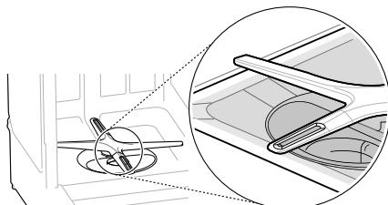
With the lower rack removed, place a level on the inside wall of the tub to check that the dishwasher is level from side to side.
