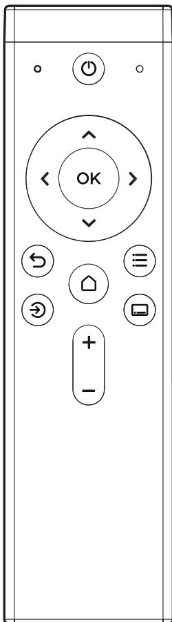
① (Standby key) Turn the TV ON or into standby mode.
