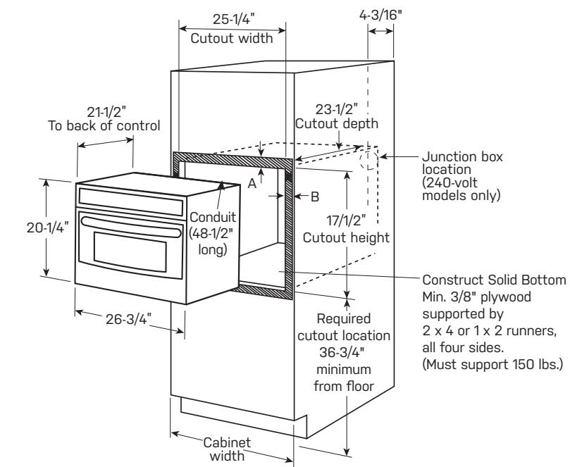
A / B = Allow the following clearances around the cutout on the front surface of the cabinet: 17/8" from the top, 7/8" from the side edges and 1 1/8" from the bottom.
