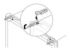
**2** Bend the tabs on the brackets to secure them to the frame using a pair of needle nose pliers.
