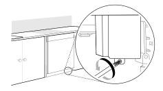
Use a Phillips screwdriver to remove 2 screws0.
