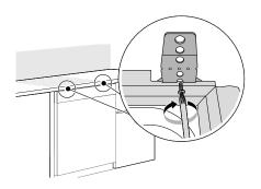
Use a nipper or tin snips to carefully trim off the excess part of the bracket.
