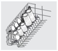
The Stemware holder is used to securely hold your wine glasses in place for the best wash. To properly secure you glass simply press the stem of the glass into the center of the Cupshelf the plastic pieces will secure around the stem to hold the glass in place.
