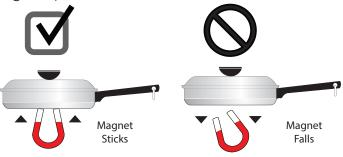
Figure 4: Magnet test
