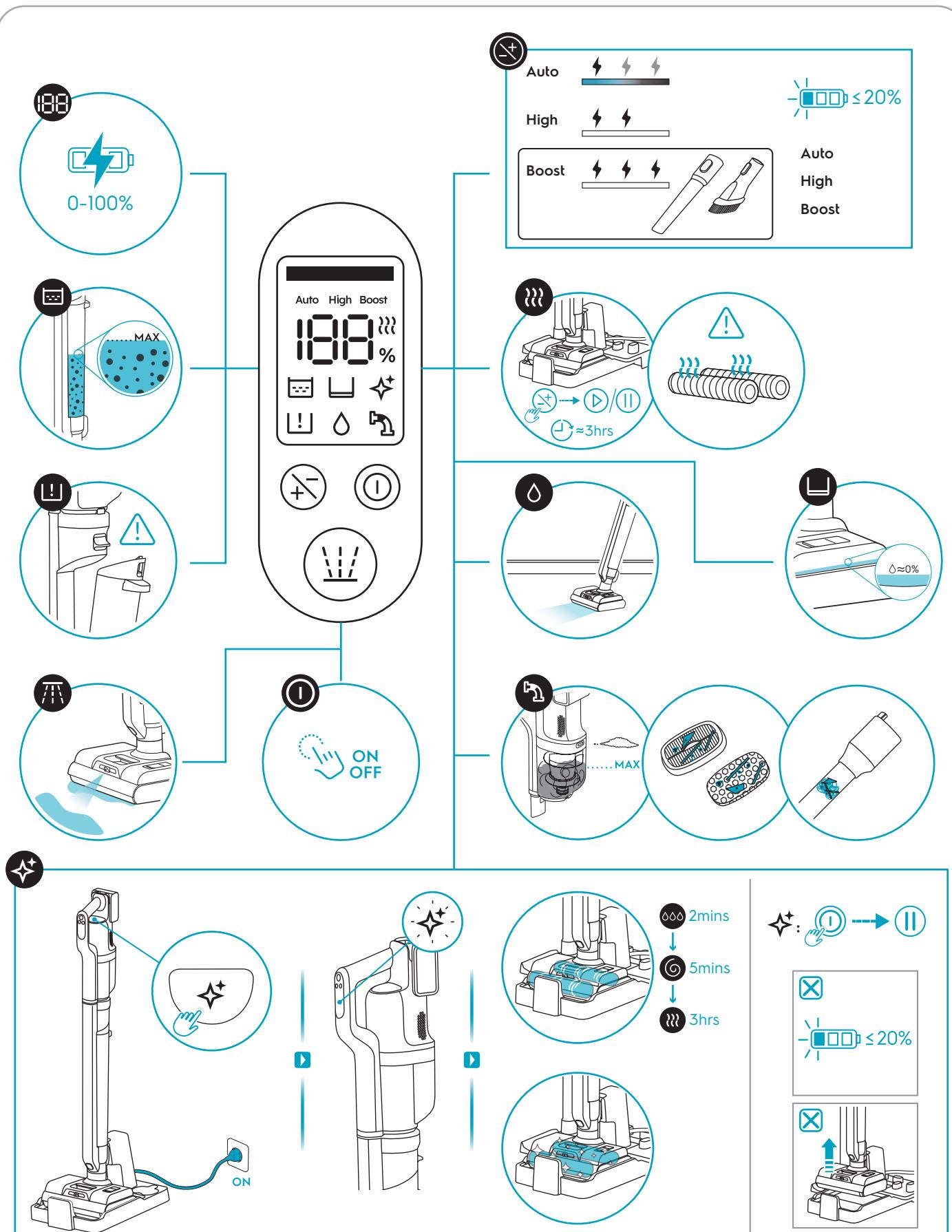
To use the self-cleaning function, the machine needs to be in the powered-on state, with the battery level greater than 20% and placed on the charging socket.
