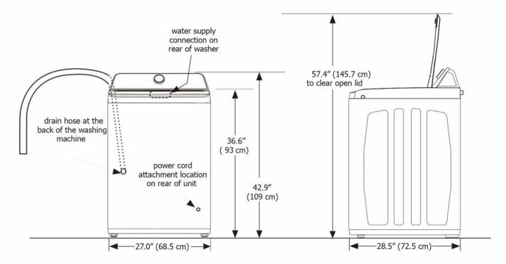
$<sup>^{\</sup>mbox{\tiny 1}}\mbox{Drain}$  hose length on washer approximately 66.93 inches (170 cm).
