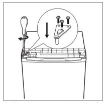
Place top cover on the back and fix with 2 screws.
