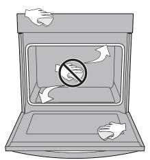
Figure 9: Clean around the oven door gasket
