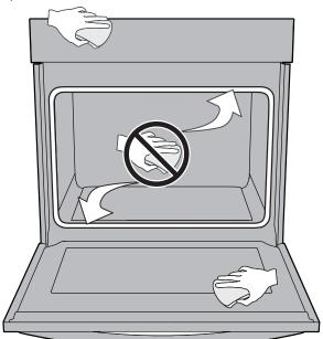
Figure 7: Clean around the oven door gasket
