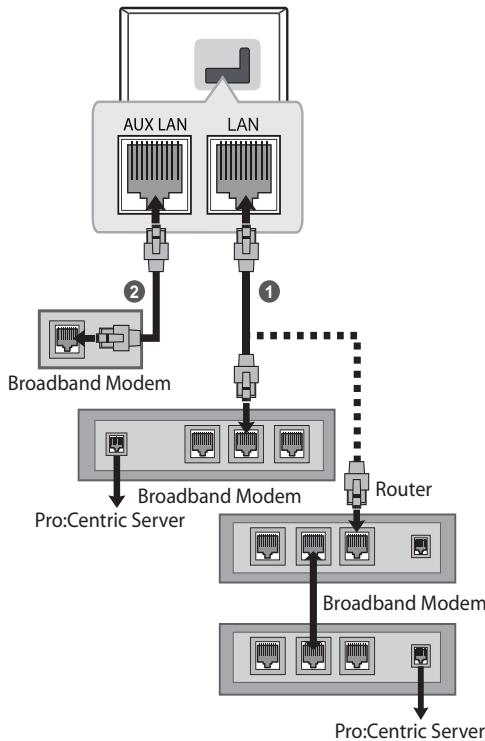
① Connect the **LAN** port of the Modem or Router to the **LAN** port on the TV.
