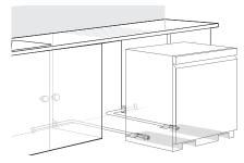
2 Smooth out or pad the edges of the hole drilled for the water supply to avoid damaging the drain hose.
