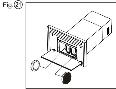
Reinstall the grease filter close aspiration plate.(fig. 21).
