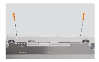
**2.** Unscrew the two Phillips screws to remove the top cover.
