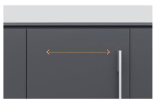
**6.** Push panel side-to-side to adjust horizontally. Ensure panels are flush with the front of the cabinet.
