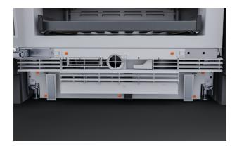
**2.** Unscrew the two Phillips screws from behind the flap and the five screws from the grille front. Set aside.
