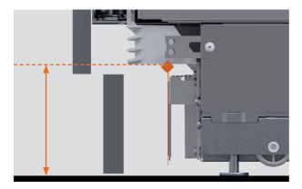
2. Measure the distance from the floor to the bottom of the grille to determine the position of the toe kick mounting plate.
