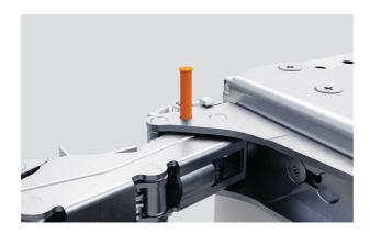
**4.** To limit the door opening to 90°, lower the hinge limiting pin into the upper and lower hinges.
