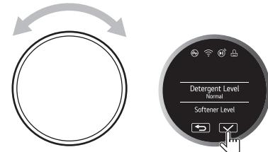
**3** Turn the knob to select **Off** and press the  $\checkmark$  button.
