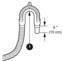
**inches (10 cm)** beyond the end of the elbow bracket, mold or microorganisms could spread to the inside of the washer.
