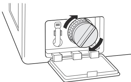
**8** Close the drain pump filter cover.
