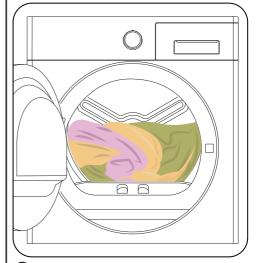
IMPORTANT: It is not recommended to load the dryer with more laundry than the amount shown in the figure. When overloaded, the drying performance of the dryer will decrease and the dryer and laundry might be damaged.
