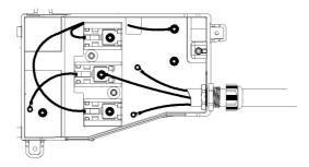
5. Connect the neutral ground conductor under the screw B. Then connect the remaining supply cord wires under the outer terminals of the block. Tighten all screws. After every connection is completed, tighten strain relief clamp in order to secure the supply cord. Finally, cover up the box cover.
