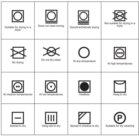
Do not dry thin, multi-layer or thick-layer fabrics together as they dry at different levels. For this reason, dry clothes together that have the same structure and fabric type. This way, you can get an even drying result. If you think that the laundry is still wet, you can select a time program for additional drying.
