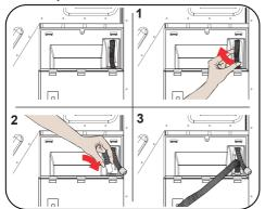
ATTENTION: The hose must be connected in a manner that it cannot be displaced. If the hose comes out during water discharge, there might be flooding in your house.
