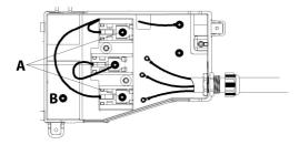
4. Remove the neutral ground conductor from central terminal and connect the neutral wire of the supply cord under the central terminal of the block. Tighten the screw.
