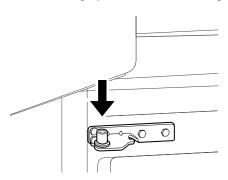
**2** Fit the hinge **1** over the hinge lever latch **2** and slot it into place. Rotate the lever 3 clockwise and fasten the hinge.
