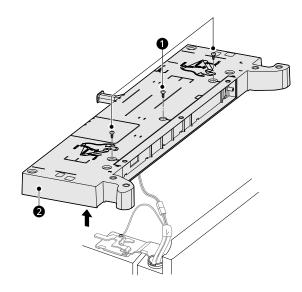
2 Remove the cover. Disconnect all wire harnesses 3 and unscrew the ground wire 4.
