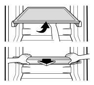
To assemble, slide the shelf into the guides until it stops.
