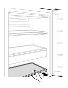
Press on the hook inside the top compartment and remove the Fresh Air Filter.
