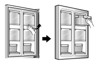
Use the handles to pull the kimchi container forward and remove it.
