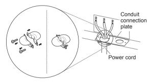
Assembling power cord strain relief at the 13/8" opening
