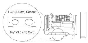
Remove the Conduit connection plate
