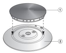
■ Place the burner cap ① on the burner base so that the lobes on the burner cap engage in the holes in the burner base.
