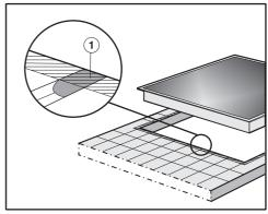
Grout lines ① and the shaded area under the cooktop frame must be smooth and even. If they are not, the cooktop will not sit flush with the countertop and the sealing strip underneath the cooktop will not provide a good seal between the cooktop and the countertop.
