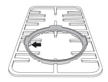
■ If you are using the wok ring, place it on the grate so that it sits securely in position and cannot move (see diagram).
